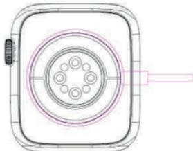
Connect the magnetic connector into the charging position as shown in the figure below, using smartphone charger 5V/1A.
